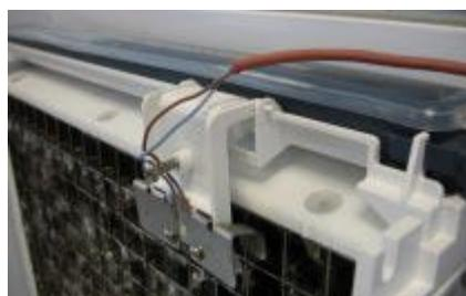
4. Disconnect the water hose from the tubing of the trough and remove the 'water trough' from its location by squeezing the retaining brackets, slide to the right and lift above the evaporator so to then clean & rinse clear of any slime or scale build up.
