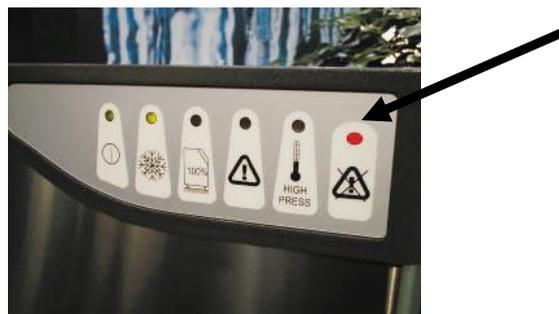
7. After approx 15 minutes (or longer if the scale build up is considered heavy), push again the **RESET BUTTON**. The P.C. Board will now put the machine into an automatic rinsing mode with the special blinking (blink twice and repeat) of the Yellow 'Bin Full' LED.
