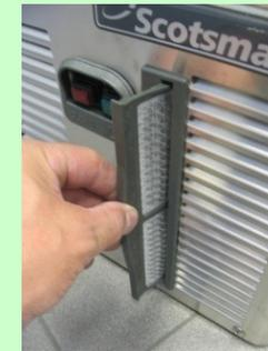
If the 'Red' LED on the front panel is flashing whilst the machine is working, it is time for a routine clean – preset at time of installation (usually set at 6 months)
