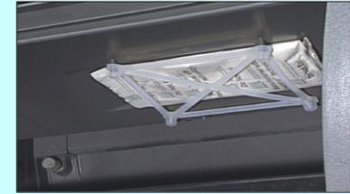
Keep grills clear of obstructions and clean regularly.....The machine requires air flow around it to operate correctly
